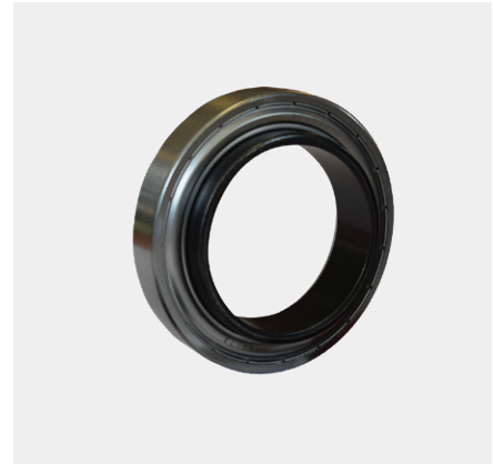
780239 PTO Release Bearing John Deere 3210 3310 3410 65mm ID 100mm OD 27mm Width OE Ref: 7700019961
