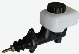
3823R Clutch Master Cylinder 50 Series Dot 4 Brake Fluid Repair Kit is 3981R OE Ref: AL66918
