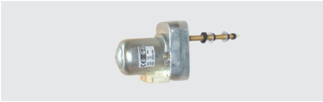
41656 Wiper Motor 12 Volt 120; Straight Single Spin Shaft Length 99mm
