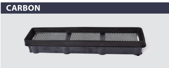
CARBON 58850 Cab Air Filter Carbon Pesticide John Deere 5320 5420 5520 5320 5420 5520 6100SE 6200SE 6400SE 6200 6300 6400 6405 6505 6506 6600 OE Ref: AL119095CA
