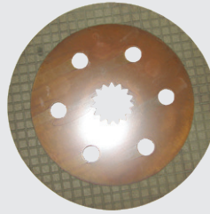
59709 Brake Disc John Deere 7600 - 7800 7600 - 7810 From S/N 007411 Teeth have square profile 15 Splines OE Ref: RE186965
