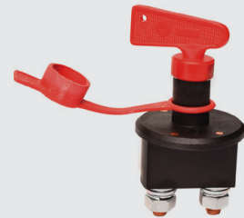
2923 Cut Off Isolation Switch - Heavy Duty Max 24V - Max 500A 5 Seconds - Max 100A
