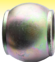
54455 Cat 2/3 Lower Link Ball 57mm OD 36.5mm ID 44.5 Width
