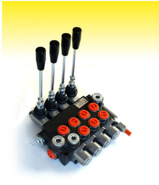
51615 Spool Valve Monoblock 1/2" BSP 4 Bank Double Acting, Double Acting, Double Acting Single Acting
