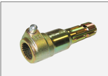
3147 Quick Release PTO Adaptor 1000 - 540 RPM 1 3/8" x 21 Splines & 1 3/8" x 6 Splines 1000 - 540 RPM
