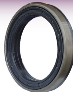
64504 Hub Seal Landini Landpower 185 4WD Inner Front Axle 70 x 95 x 13/14.5 OE Ref: 04402311
